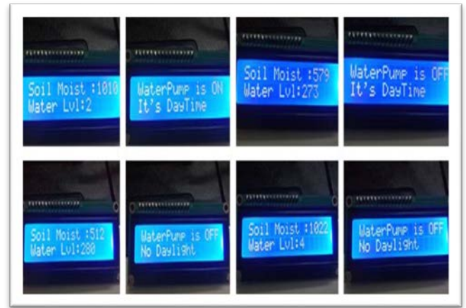
Figure 13 Sensor values and water Pump status displaying in LED
